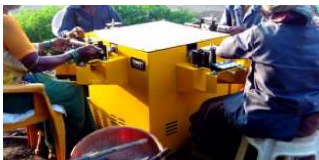
Fig 1: Sugarcane Bud Cutter: A Sugarcane Bud Cutter Is Used To Cut the Buds (Eye) of the Sugarcane Which Can Be Used As Seeds for Plantation Purposes
