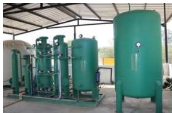
Biogas to Bio-CNG Purification Unit:- Adsorption Filter System for Removal of H 2 S, CO 2 , and other impurities gases
