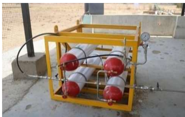
Bio-CNG Two Cascade Set: - 1.4 X 13.5 Kg = 54 Kg, 2.3 X 9.7 kg = 29.1 Kg
