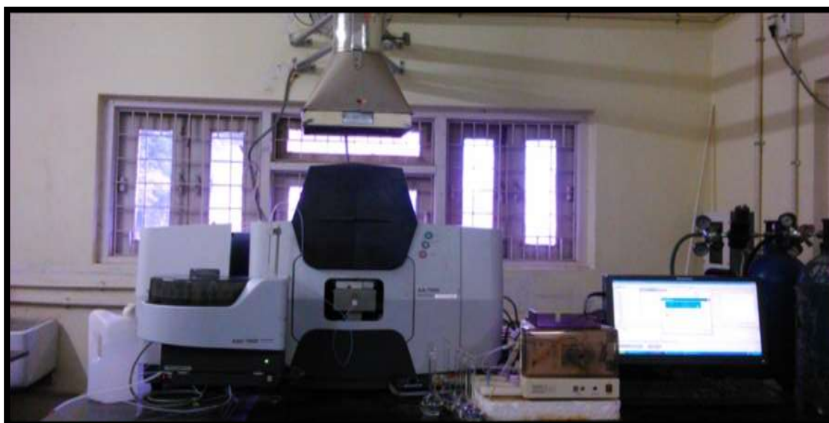
Fig 5: Analysis of soil and plant samples through Atomic Absorption Spectrophotometer
