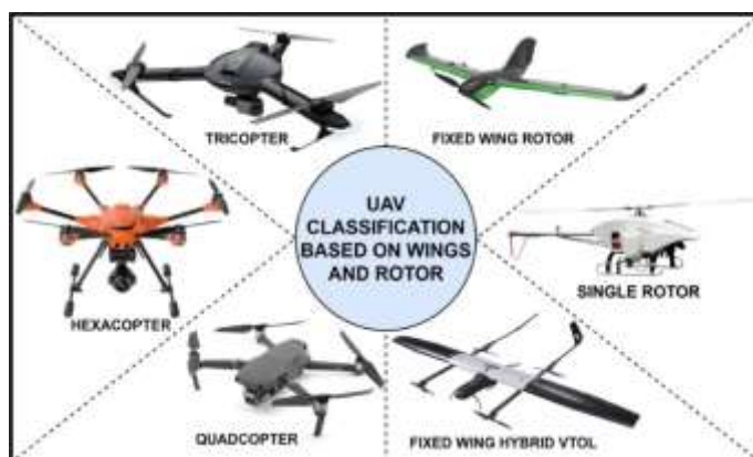
Fig 2: UAV Classified on the Basis of Wings and Rotor
