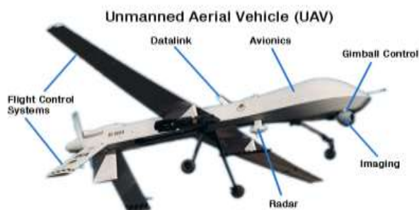
Fig 3: Unmanned Aerial Vehicles with its Parts
